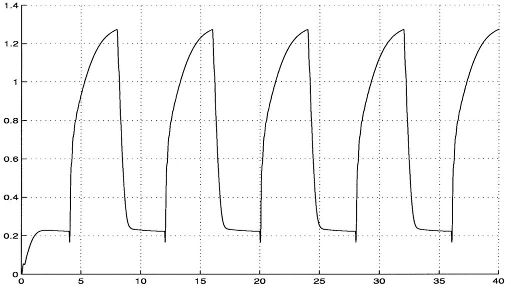
Fig. 7. NN weight  $\|\hat{V}\|_F$  (state feedback).
