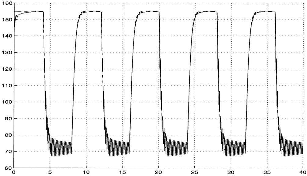
Fig. 11.  $u$  follow IDFC  $u_d$  ("--") (output feedback).
