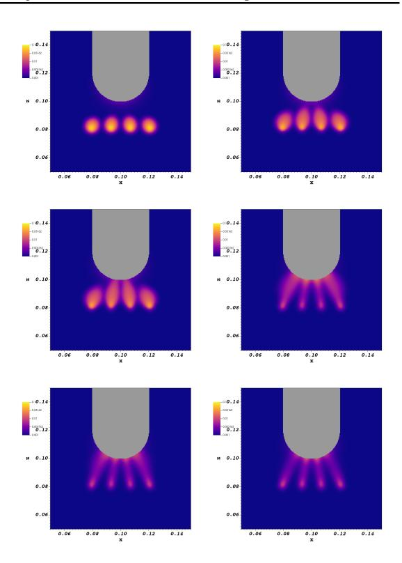
Figure 4.27: Cross section of electron density  $n_e$  at y = 0.1. Six subfigures are depicted at time t = 0.37, 0.77, 0.97, 2.40, 3.02 and 3.83 (ns), ordered from left to right and top to bottom.
