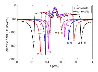
Figure 2.6: Electric field  $E_z$  along the line x = 0.5, y = 0.5 in a double-headed streamer (reference data taken from [14]).
