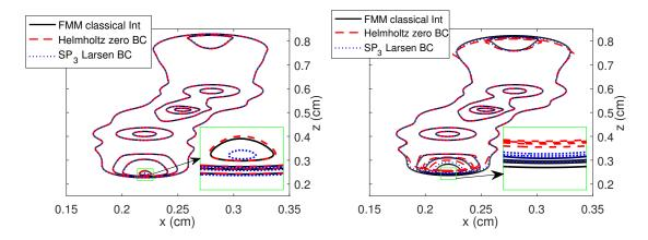
Figure 3.13: Contours of different electron density values at  $n_e = 1 \times 10^{13}$ ,  $5 \times 10^{13}$ ,  $9 \times 10^{13}$ ,  $1.3 \times 10^{14} \text{ cm}^{-3}$ , on plane y = 0.25 cm at 1.5 ns for  $p_{o_2} = 150 \text{ Torr}$  (left) and  $p_{o_2} = 1 \text{ Torr}$  (right).
