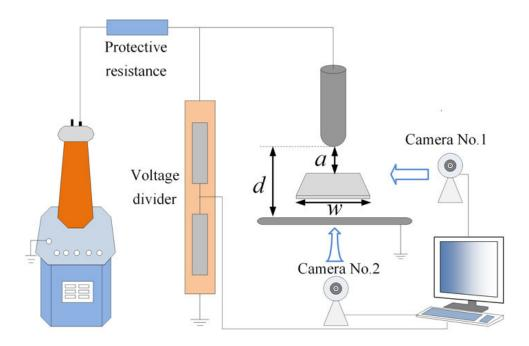
Figure 1.3: Schematic diagram of the experimental setup. Reprinted from [180] with permission.
