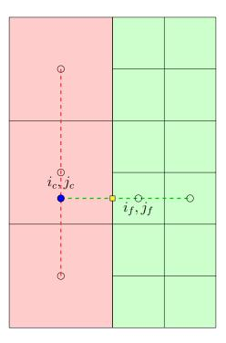
Figure 4.16: Some regular cells in two AMR levels for quadratic interpolation to construct the left flux of  $(i_f, j_f)$ . Quadratic interpolation is first applied along the red dashed line to evaluate the value at blue solid circle. Then this solid value together with two values at fine level along with the green dashed line constructs the gradient at the yellow solid square.
