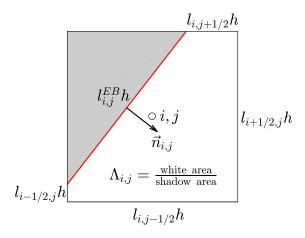
Figure 4.5: Geometry notations of an irregular cell.
