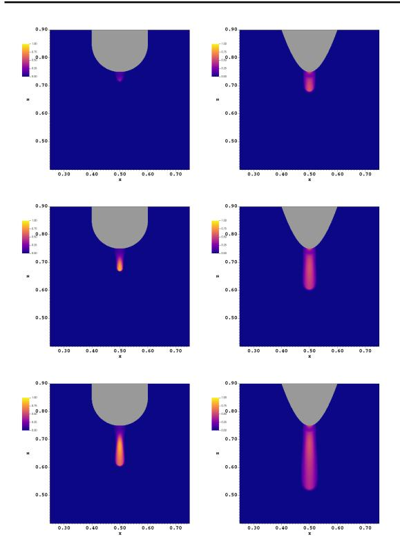
Figure 4.22: Cross section of electron density  $n_e$  on plane y = 0.5 at three different times t = 3, 6, 9 (ns). (ordered from top line to bottom line). Left subfigures: round-rod anode; right subfigures: hyperbolic anode.
