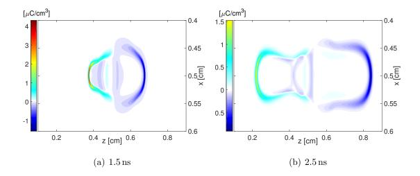
Figure 2.8: Net charge density (in terms of charge per unit volume) on the y = 0.5planes in a double-headed streamer at 1.5 and 2.5 ns. Here net charge density equals to the density of the charge carriers  $(n_p - n_e)$  times the elementary charge  $(1.602 \times 10^{-13} \mu \text{C})$ .
