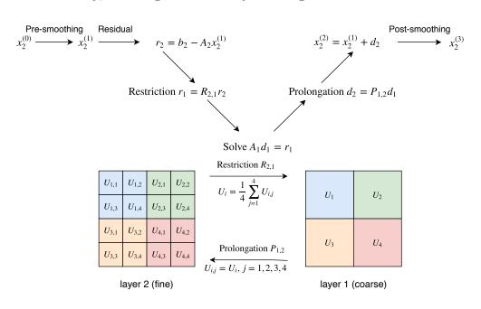
Figure 2.1: Diagram of V-cycle geometric multigrid for uniform mesh in two layers.
