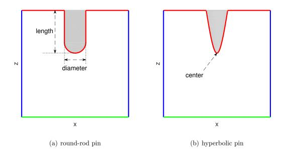
Figure 4.1: Cross sections of two typical examples of simulation domain  $\Omega$ . The shadow part is outside simulation.
