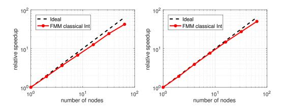
Figure 3.15: Relative speedups over two meshes:  $256 \times 256 \times 160$  (left) and  $512 \times 512 \times 320$  (right). 20 cores are used in each node.
