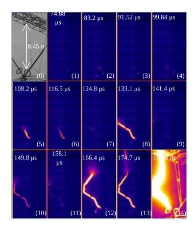
Figure 1.2: The time-resolved photographs of discharge development in a conductortower lattice. Reprinted from [29] with permission.
