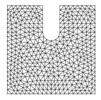
Figure 4.2: Unstructured grid of 2D domain from the cross section in Figure 4.1(a).
