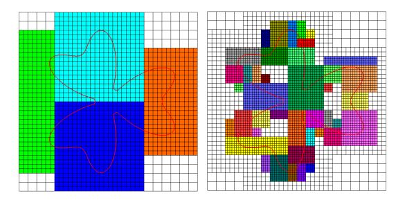
Figure 4.14: The AMR grid in Figure 4.13 with different dyed patches in the second layer (left subfigure) and the third layer (right subfigure).
