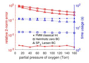
Figure 3.10: Error (red color, solid line) and time usages (blue color, dotted line) of FMM classical Int, Helmholtz zero BC and  $SP_3$  Larsen BC methods with different air pressures.
