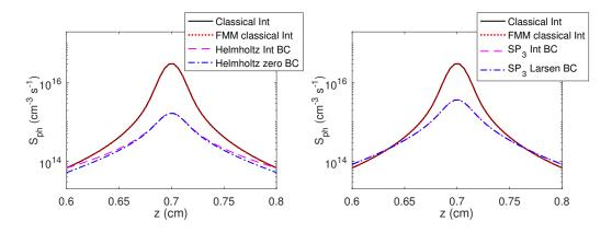
Figure 3.9: Photoionization rate  $S_{\rm ph}$  along line x = y = 0.125 cm, calculated from one Gaussian in (3.25) with  $p_{o_2} = 10$  Torr.
