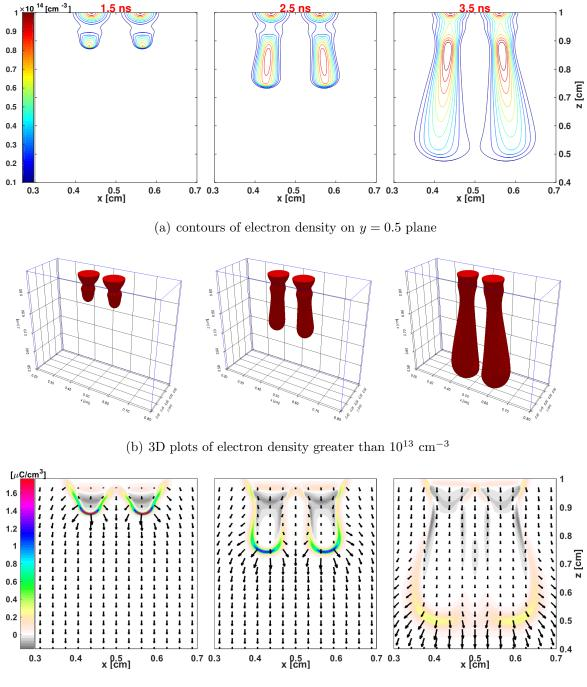
(c) net charge density and electric field  $(E_x, E_z)$  on y = 0.5
