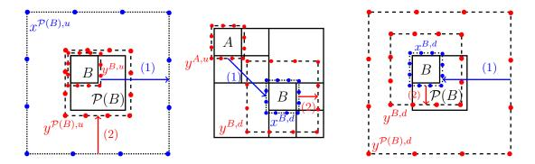
Figure 3.4: Cross section of M2M translation (left subfigure), M2L translation (middle subfigure) and L2L translation (right subfigure). Dashed lines with red dots denote equivalent surfaces. Dotted lines with blue dots denote check surface. Step (1) in blue arrow is the evaluation of potential on check surface, and step (2) in red arrow is the calculation of equivalent density on equivalent surface.  $\mathcal{P}(B)$  denotes parent box of B.
