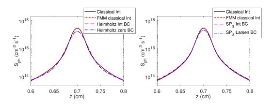
Figure 3.8: Photoionization rate  $S_{\rm ph}$  along line x = y = 0.125 cm, calculated from one Gaussian in (3.25) with  $p_{o_2} = 160$  Torr.
