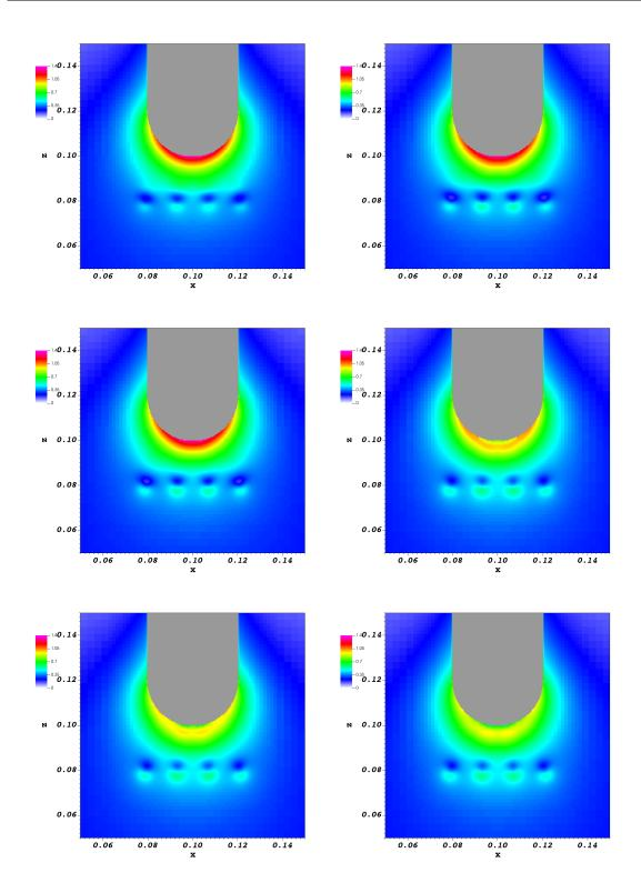
Figure 4.28: Cross section of magnitude of electric field  $|\vec{E}|$  at y = 0.1. Six subfigures are depicted at time t = 0.37, 0.77, 0.97, 2.40, 3.02 and 3.83 (ns), ordered from left to right and top to bottom.
