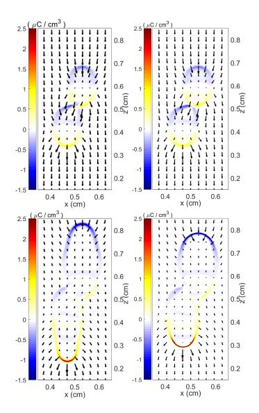
Figure 3.12: The net charge density and the electric field  $(E_x, E_z)$  on the y = 0.5 plane at t = 0.5 ns (top row) and t = 1.5 ns (bottom row). The subfigures in the left column are simulation results with photoionzation, while the subfigures in the right column are results without photoionization.
