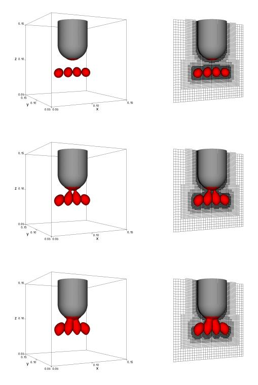
Figure 4.25: Left subfigures: the contour surfaces (red color) of electron density  $n_e = 0.002$  at three different times t = 0.37, 0.77, 0.97 (ns). Right subfigures: slices of mesh at y = 0.1 of the corresponding left subfigures.
