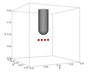
Figure 4.24: Simulation domain and initial condition. The round-rod pin is dyed as gray color, and contour surface of electron density 0.01 is dyed as red color.
