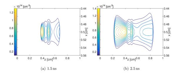
Figure 2.7: Electron density on the y = 0.5 plane in a double-headed streamer at 1.5 and 2.5 ns.
