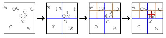
Figure 3.1: An example of a hierarchical tree in 2D, with  $N_{\rm pt} = 10$ , m = 2. The arrows show the construction procedure, and the circles with "+" denote the  $N_{\rm pt}$  points.
