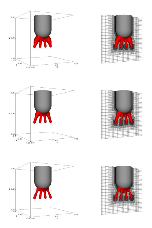
Figure 4.26: Left subfigures: the contour surfaces (red color) of electron density  $n_e = 0.002$  at three different times t = 2.40, 3.02 and 3.83 (ns). Right subfigures: slices of mesh at y = 0.1 of the corresponding left subfigures.
