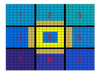
Figure 2.2: Explanation of communication for  $n_e$ ,  $n_p$  in a 2D case.
