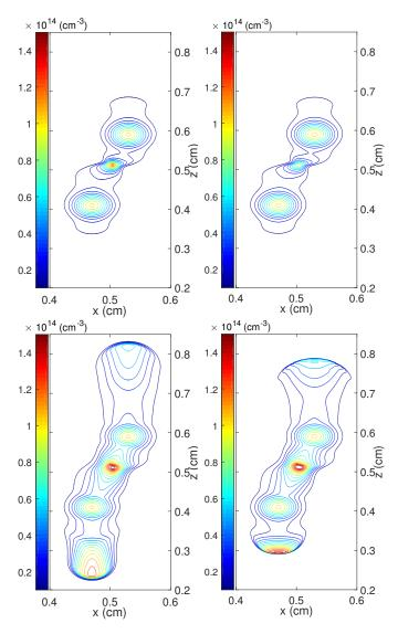
Figure 3.11: The contour of electron density on the y = 0.5 plane at t = 0.5 ns (top row) and t = 1.5 ns (bottom row). The subfigures in the left column are simulation results with photoionzation, while the subfigures in the right column are results without photoionization.
