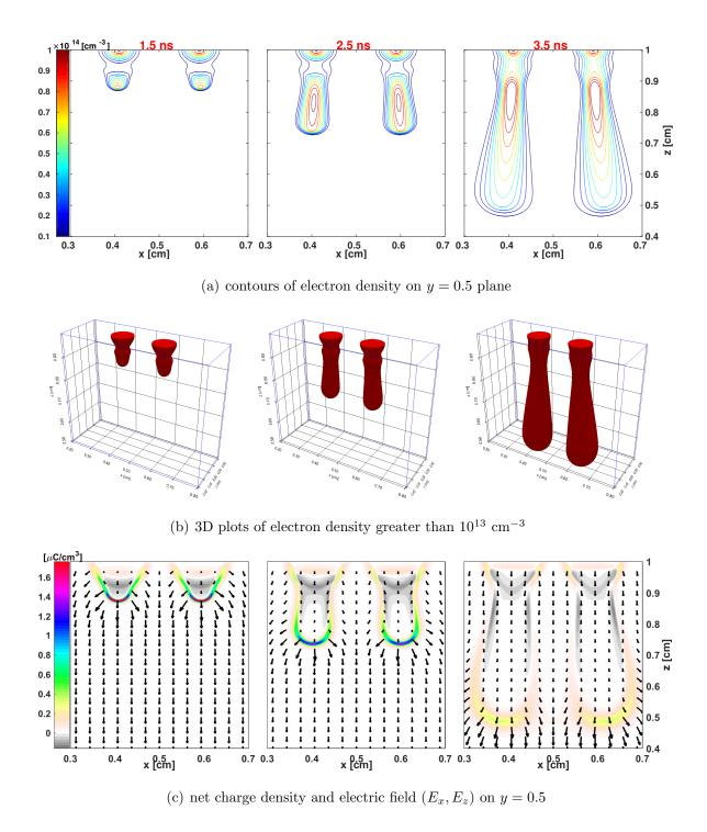
Figure 2.11: Electron density, net charge density and electric field  $(E_x, E_z)$  for the interaction between two streamers for  $x_0 = 3\sigma$ .
