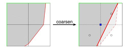
Figure 4.10: Illustration of coarsening procedure. Four finer cells combine to one coarser cell centered at blue square. The coarser value is taken as the volume-weighted average of all three non-covered finer value centered at circles. The red solid line in the right subfigure shows the EB edge of this coarser cell.
