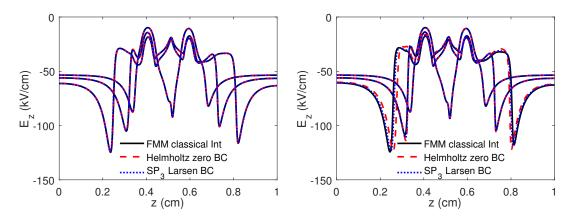
Figure 3.14: The third component  $E_z$  of the electric field  $\vec{E}$  along line x = y = 0.25 cm, at 0.5, 1.0 and 1.5 ns for  $p_{O_2} = 150 \text{ Torr}$  (left) and  $p_{O_2} = 1 \text{ Torr}$  (right).
