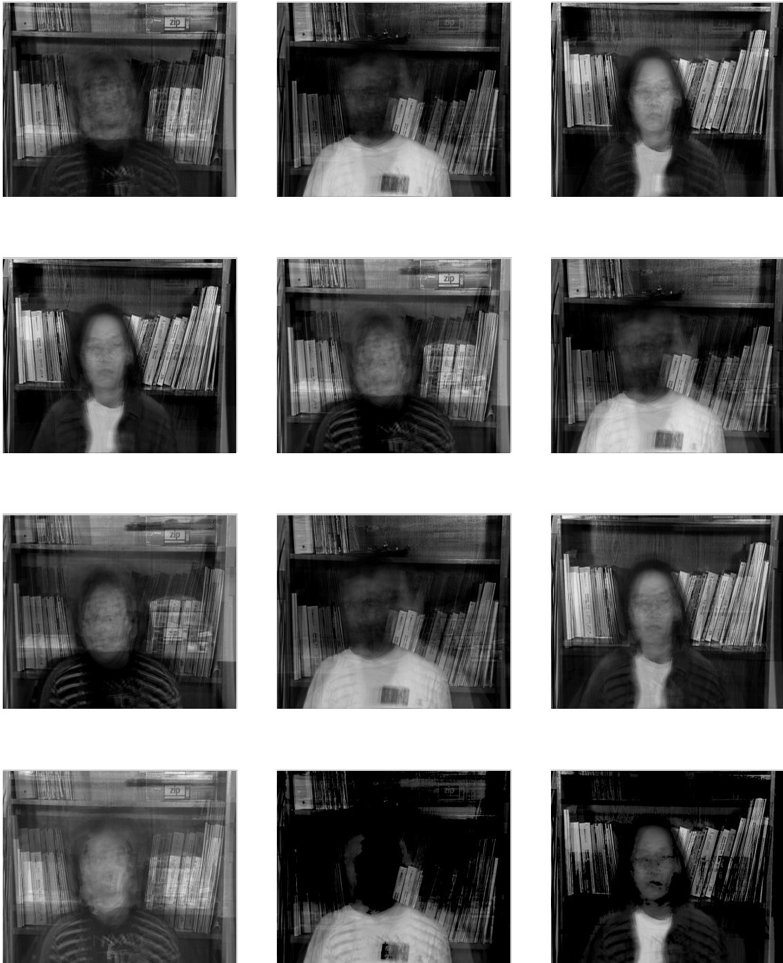
Figure 3.7: Basis images of 3 individuals in Georgia Tech dataset obtained at the 20 th iteration. The first to fourth rows pertain to rand , cr1-nmf , spkm , and nndsvd initializations respectively.
