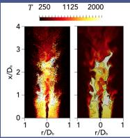
Instantaneous turbulent temperature fields in a swirl flame by a sparse stochastic Monte Carlo method (left) and a finite volume method (right).
