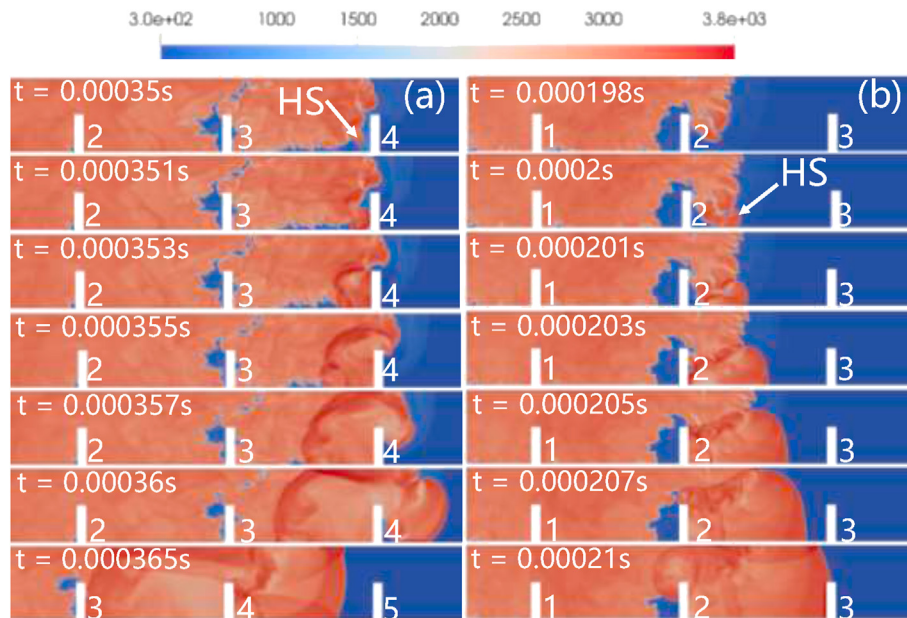
Fig. 9 – Time sequence of temperature (in Kelvin) distributions of the stoichiometric \text{NH}_3/\text{H}_2/\text{O}_2 mixture with \text{NH}_3/\text{H}_2 molar ratio \alpha = (a) 1:1 and (b) 1:2.
