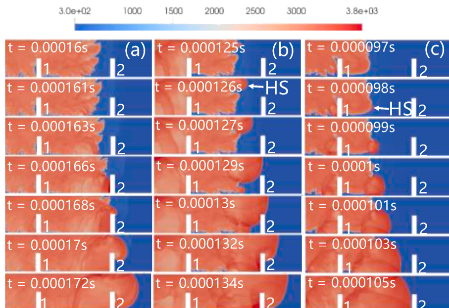
Fig. 10 – Time sequence of temperature (in Kelvin) distributions of the stoichiometric \text{NH}_3/\text{H}_2/\text{O}_2 mixture with \text{NH}_3/\text{H}_2 molar ratio \alpha = (a) 1:3, (b) 1:7 and (c) no ammonia.
