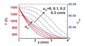
Fig. 10. Temperature (red solid lines) and OH mass fraction (blue dash-dotted lines) profiles along the vertical direction starting from the rear stagnation point for  $u_{in}=0$  m/s, 0.1 m/s, 0.2 m/s and 0.3 m/s at t=4 ms.  $T_P = 1400$  K.
