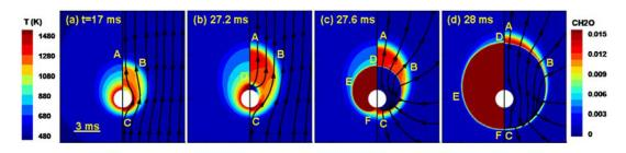
Fig. 6. Evolution of the temperature (left) and CH<sub>2</sub>O mass fraction (right) contours for  $T_P = 1400$  K and  $u_{in} = 0.15$  m/s. The filled white circle represents the hot particle with radius of 1 mm. The streamlines are imposed on contours of CH<sub>2</sub>O mass fraction. Curves ABC and DEF represents the cool and hot flames, respectively.
