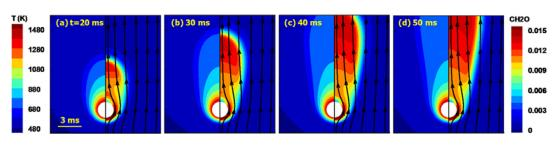
Fig. 8. Evolution of the temperature (left) and CH<sub>2</sub>O mass fraction (right) contours for  $T_P = 1400$  K and  $u_{in} = 0.3$  m/s. The streamlines are imposed on contours of CH<sub>2</sub>O mass fraction.
