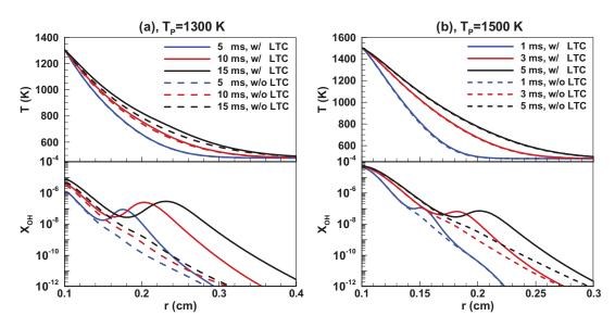
Fig. 4. Temperature and mole fraction of OH profiles for (a)  $T_P = 1300$  K and (b)  $T_P = 1500$  K. Solid and dashed lines correspond to cases with and without LTC, respectively.
