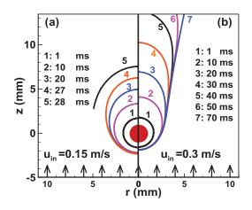
Fig. 7. Evolution of the cool flame front (iso-surface of T = 600 K) for (a)  $u_{in} = 0.15$  m/s and (b)  $u_{in} = 0.3$  m/s with  $T_P = 1400$  K. The filled red circle represents the hot particle with radius of 1 mm.
