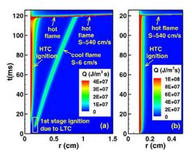
Fig. 2. Contour of total heat release rate in *r*-*t* space for (a)  $T_P = 1200$  K with LTC, and (b)  $T_P = 1425$  K without LTC.
