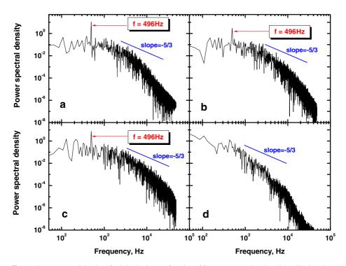
Fig. 17 Power spectral density of axial velocity as a function of frequency at various locations. The locations have been marked in Fig. 2
