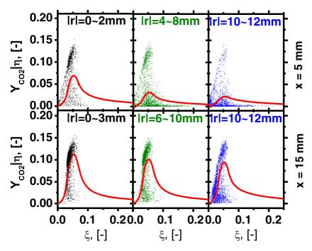
Fig. 15 Conditional CO<sub>2</sub> mass fraction at two streamwise stations x = 5 mm (first row) and 15 mm (second row) for different radial sections. Lines: time and spaceaveraged conditional temperature from LES/CMC; scatters: single-pulsed experimental data [13]
