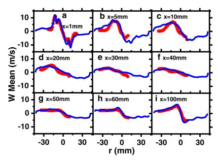
Fig. 6 Radial profiles of mean swirl velocity. Lines: LES/CMC; symbols: experimental data from Ref. [14]
