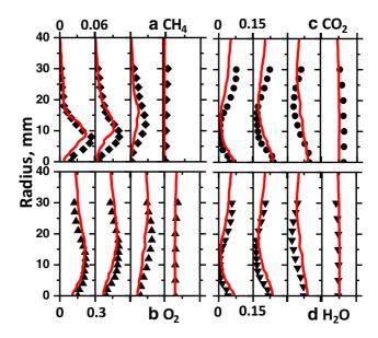
**Fig. 12** Radial profiles of time-averaged mass fractions of (a)  $CH_4$ , (b)  $O_2$ , (c)  $CO_2$  and (d)  $H_2O$ . Legend as Fig. 5. Streamwise locations for four sub-figures (left to right): x = 5, 10, 15 and 40 mm
