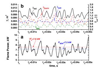
**Fig. 16** Timeseries of **a** is volume integrated heat release rate  $(\dot{Q})$  and extinguishing factor  $(f_{ext})$  as well as **b** is areas of stoichiometric mixture fraction iso-surface  $(\Sigma_{tot}, \Sigma_{burn} \text{ and } \Sigma_{ext})$ .  $P_{th}^a$  is flame power estimated from fuel LHV, while  $P_{sim}$  is the time averaged  $\dot{Q}$  based on the shown timeseries in **a**
