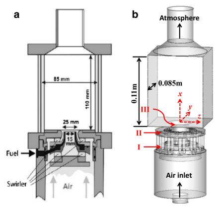
**Fig. 1** Dual swirler burner [13, 14, 19]: **a** schematic and **b** computational domain. I: inner swirler; II: outer swirler; III: fuel injectors
