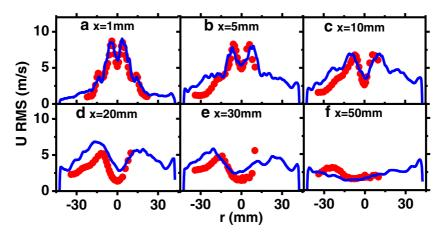
Fig. 7 Radial profiles of axial RMS velocity. Lines: LES/CMC; symbols: experimental data from Ref. [14]
