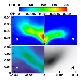
Fig. 3 Comparisons of  $\bf a$  time-averaged OH mass fraction and  $\bf b$  heat release rate (in MJ/m<sup>3</sup>s) respectively with  $\bf c$  time-averaged OH-PLIF [14] and  $\bf d$  OH\* chemiluminescence [19]. Color bar only for  $\bf a$  and  $\bf b$
