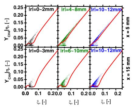
Fig. 14 Conditional CH<sub>4</sub> mass fraction at two streamwise stations x = 5 mm (first row) and 15 mm (second row) for different radial sections. Lines: time and spaceaveraged conditional temperature from LES/CMC; scatters: single-pulsed experimental data [13]
