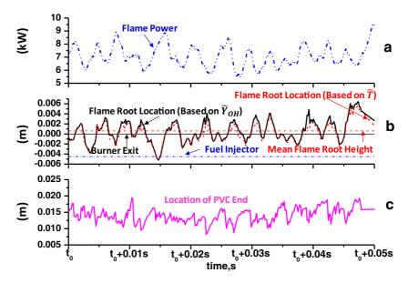
Fig. 19 Timeseries of a flame power, b flame root streamwise location and c streamwise location of the PVC end over the same period (from  $t_0$  to  $t_0 + 0.05$  s) as in Fig. 16
