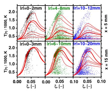
Fig. 13 Conditional temperature at two streamwise stations x = 5 mm (first row) and 15 mm (second row) for different radial sections. Thick lines: time and spaceaveraged conditional temperature from LES/CMC; thin lines: instantaneous conditional filtered temperature; scatters: single-pulsed experimental data [13]
