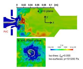
Fig. 18 PVC visualized by iso-surface of pressure (p = 101200 Pa) for **a** side view at z = 0 plane and **b** top view at z = 0.004 m plane. The iso-lines are stoichiometric mixture fraction  $\xi_{st} = 0.055$
