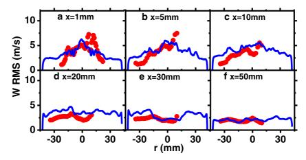
Fig. 8 Radial profiles of swirl RMS velocity. Lines: LES/CMC; symbols: experimental data from Ref. [14]
