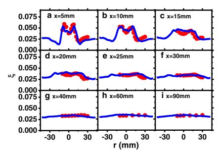
Fig. 9 Radial profiles of mean mixture fraction. Lines: LES/CMC; symbols: experimental data from Ref. [14]
