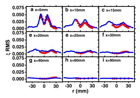
Fig. 10 Radial profiles of RMS mixture fraction. Lines: LES/CMC; symbols: experimental data from Ref. [14]
