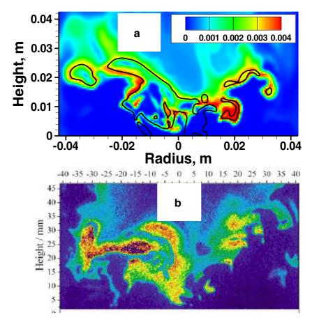
Fig. 4 Instantaneous a filtered OH mass fraction and b OH-PLIF [14]. Isolines in (a):  $\xi_{st} = 0.055$
