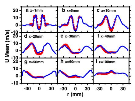
Fig. 5 Radial profiles of mean axial velocity. Lines: LES/CMC; symbols: experimental data from Ref. [14]
